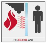
This type of glazing can typically be used where building codes require an assembly designated "fire resistant" to enclose a space.
