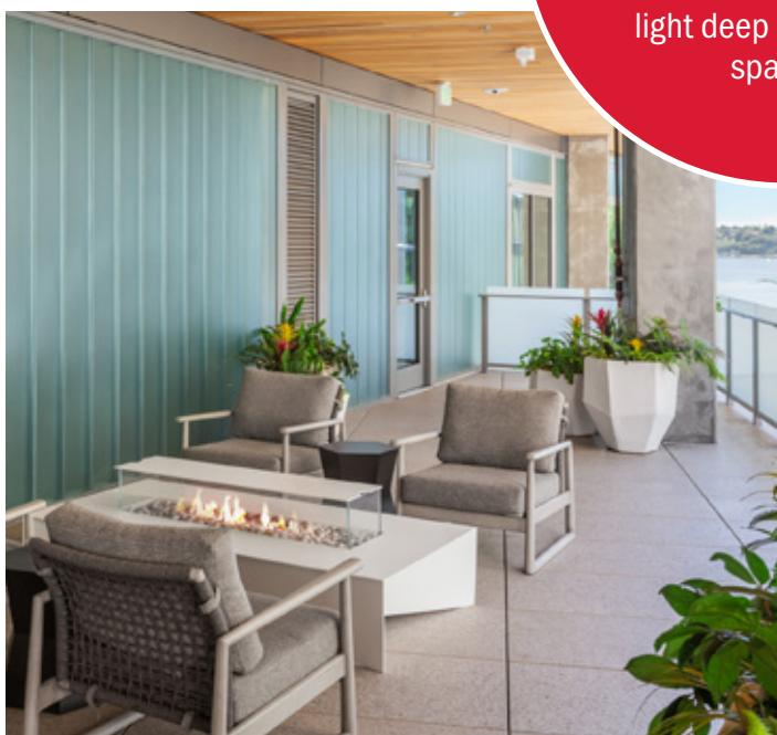
The self-supporting, U-shaped, linear cast-glass channels and extruded perimeter frame allow for large, glazed areas that can diffuse extensive amounts of natural light deep into interior spaces.
